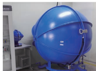
Integrating Sphere (for Testing LED Luminous)
