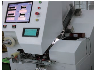
3 in 1 Auto inspection machine (Flatness/ Visual/ Taping)
