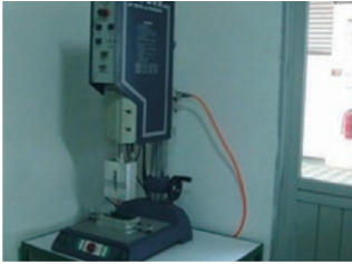
Ultrasonic Welding for Sealing Plastic Case
